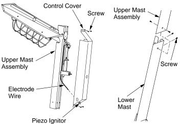
Figure 7 - Removing Control Cover
